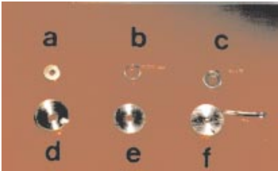
Figure 5 The parts of the DS retractor: (a) drum, (b) constant force spring (CFS), (c) CFS mounted on the drum, (d) spring box (SB), (e) spring cover and (f) DS retractor.
